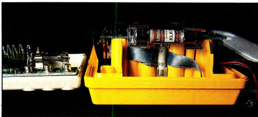
Note the difference in meter protection. The heavy-duty meter has both a 10A and 2A fuse, while the smaller meter has only a 0.8A fuse.
