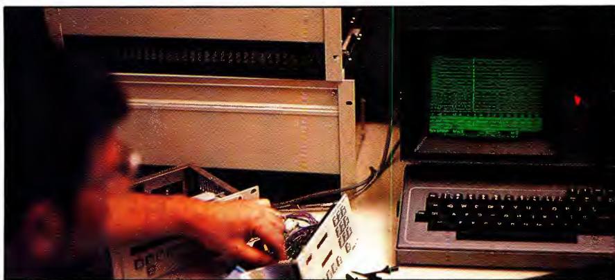
Logic analyzer is shown connected to a routing switcher for troubleshooting.
